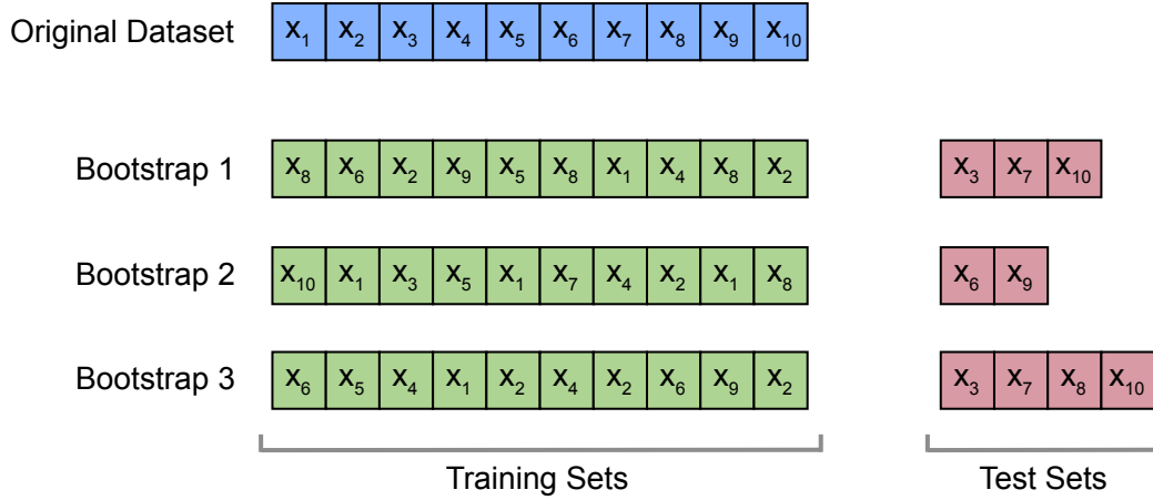
Figure 7: Illustration of training and test data splits in the Leave-One-Out Bootstrap (LOOB).
